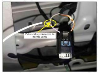
13.Unplug the tailgate pulse cable socket (The button of the original car open trunk). Our pulse cable connects to this purple cable).
