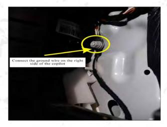
10. Find the ground wire on the right side of the copilot and connect the ground wire.
