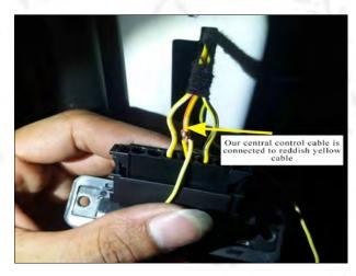
12.Our central control cable is connected to the reddish yellow cable of this seat (The third hole in the first row from left to right)
