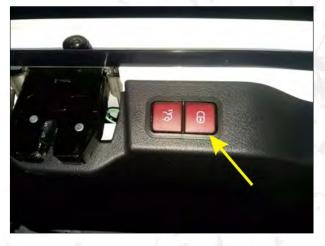
19.Cut a small square with the blade at the original tailgate trim panel and install our tailgate switch button.
