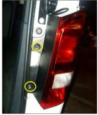
6.Remove the two screws in the yellow circle and remove the car lights (The left and right steps are the same).
