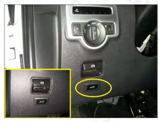
8.Remove the trim panel from the main driving, punch holes and install our front switch button.
