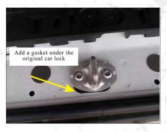
17. Remove the original car lock and add a gasket under the original car lock.
