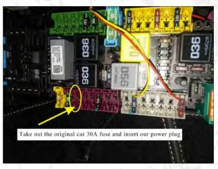
9.Remove the trim panel under the copilot to find the power supply, unplug the original car 30A fuse. Plug in our power plug.
