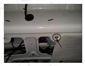
18.Insert the brace rod socket, electric suction lock socket and power cord socket into the control box. Central control box installation position. Fixed the central control box with the original car screws, meson and gasket.
