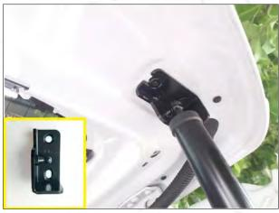
3.Remove the original right upper bracket and the brace rod. Install our upper right bracket (The ball head position is facing outward). and fix it with our screws.
