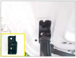
5.Remove the original left upper bracket and the brace rod. Install our upper left bracket (The ball head position is facing outward). and fix it with our screws.
